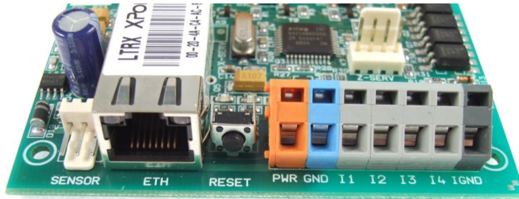
Fig. 6 – example of terminals on Quido ETH 4/4 (from left): sensor, ethernet, power supply and inputs
