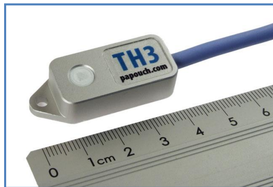
Fig. 3 – Integrated sensor for temperature and humidity
