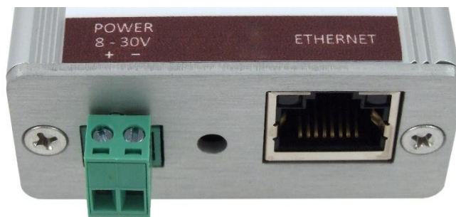
Fig. 3 – terminals for power and Ethernet connection; reset button in the middle
