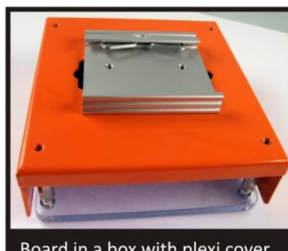
Board in a box with plexi cover and DIN rail mount (bottom)
