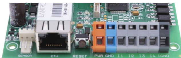
Fig. 6 – example of terminals on Quido ETH 4/4 (from left): sensor, ethernet, power supply and inputs
