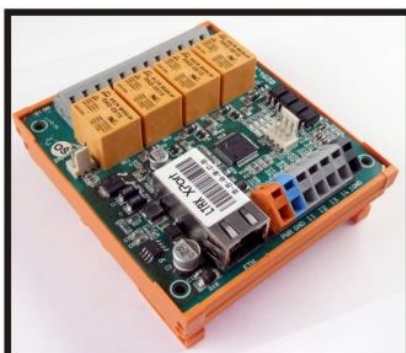
Board with a DIN rail
