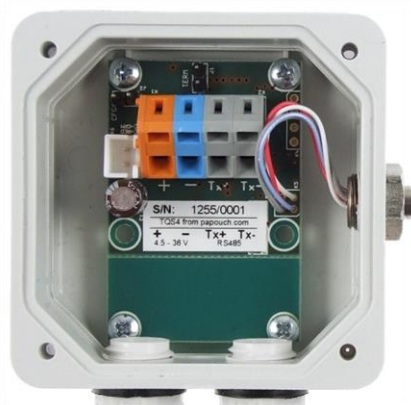
fig. 2 – Terminal block inside the box
